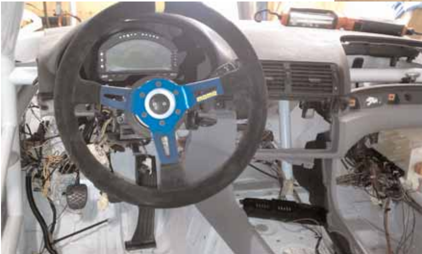
Trimmed wiring harness being threaded into its new home.
