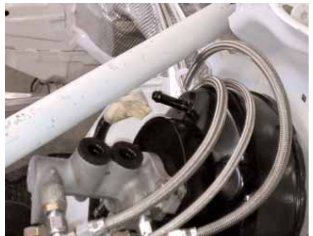
Custom fit brake booster. Adapters and machining by Geoff Atkinson.
