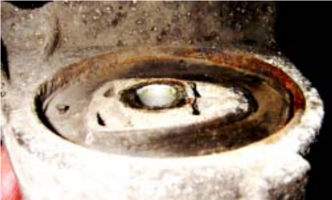
Photo #3 Bushing that "walked." through bolt. Oh yeah, and put a new o-ring under that speedometer sensor!
