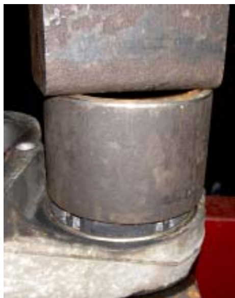
Photo #2 Bushing pressed into place.
