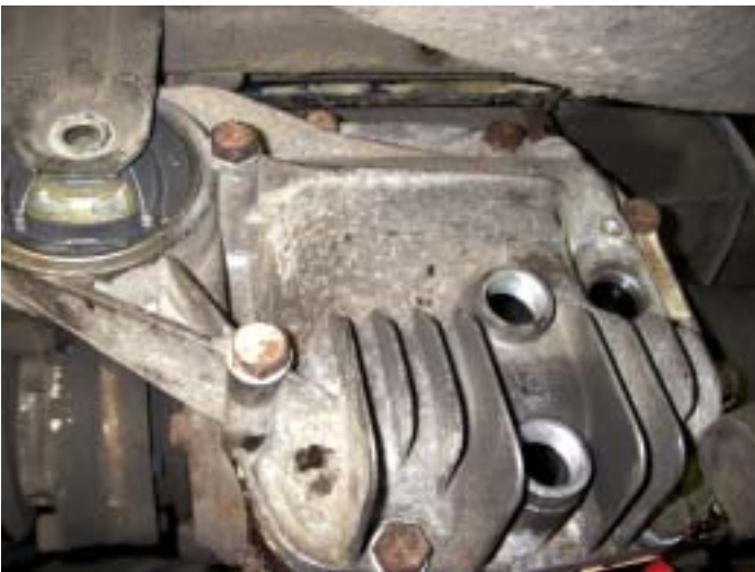
Photo #4 Re-installed diff cover.
