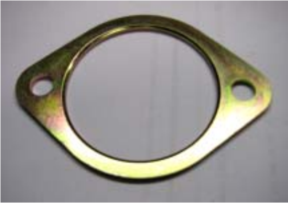
Photo #2 Reinforcement Plate for shock tower
