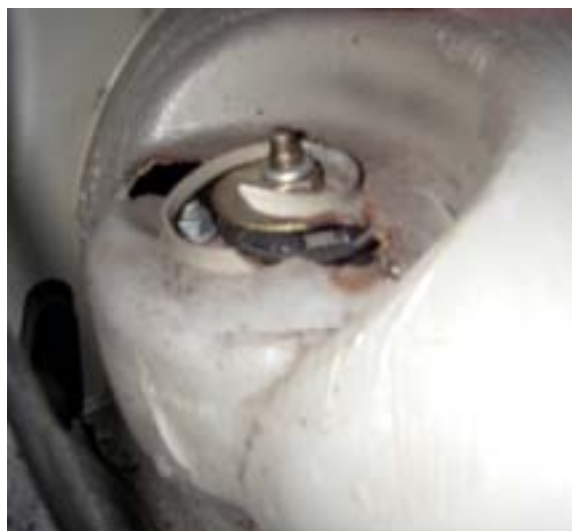
Photo #1 Failed shock tower on E36
