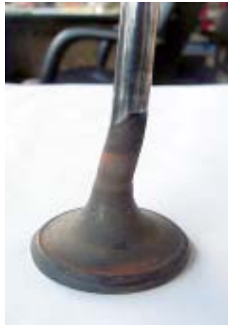
Bent exhaust valve - ouch!
