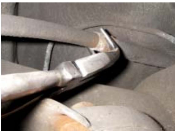
Photo #4 Extracting The Cable Sheath
