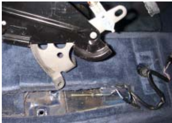
Photo #1 Removed Parking-Brake Handle
