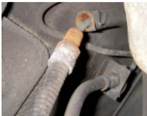
Photo #3 Cable Sheath Connection To Car Body
