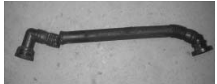
Photo #3 M54 Breather Hose Removed (2001 530i)
