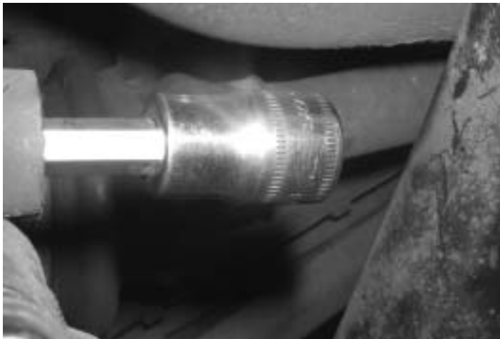
Photo #1 - Hex Bit is too long.
