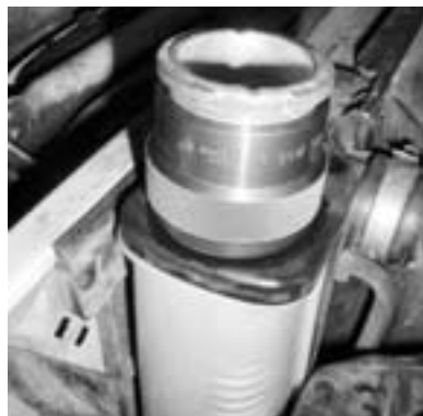
Photo #1 Pressure Test Adapter Vic Lucariello, Sr.
