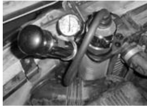
Photo #2 Pressure Tester in Action Vic Lucariello, Sr.
