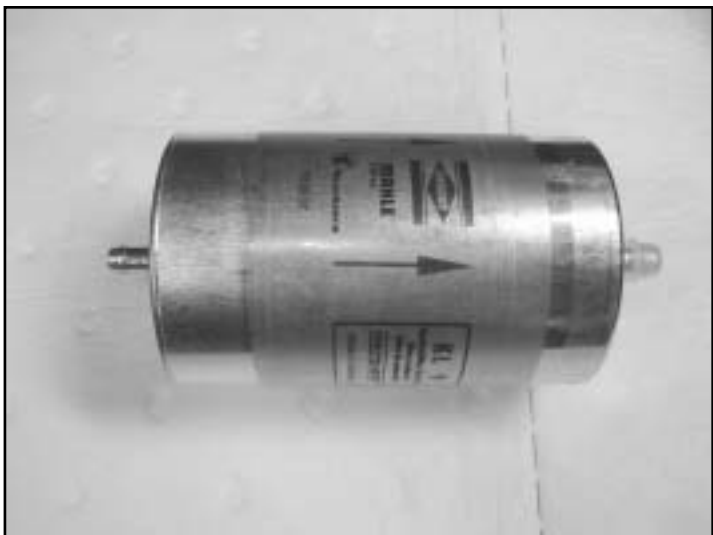
Photo 3: Note Direction-Of-Flow Arrow
