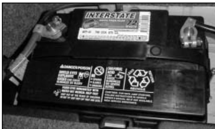
Photo 3: E36 Replacement Battery With Vent Hose
