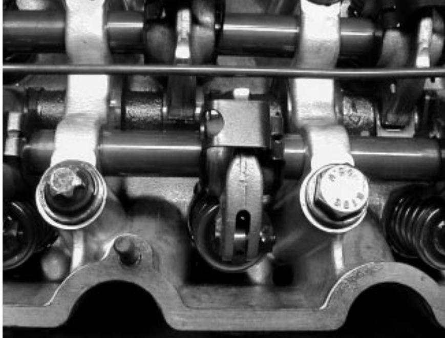
Photo 1: New type headbolt on left, old on right.
