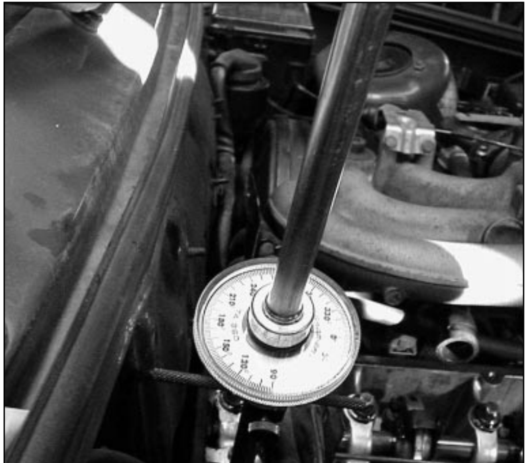
Photo 3: Tightening with a torque-angle gauge.
