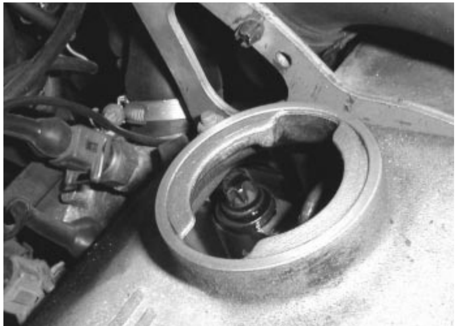
Photo 2: Determining the type of headbolt installed.
