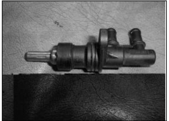
Photo 2: Valve Removed From Housing.
