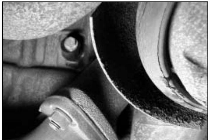
Photo 3: Engine Block Drain Plug Located On The Lower Rear Passenger Side Of The Block
