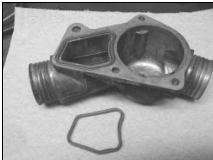
Photo 4: Be Sure To Replace The Profile Gasket When Changing The Thermostat.
