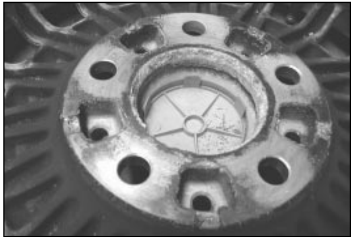
Photo 4: Corroded wheel mounting surface
