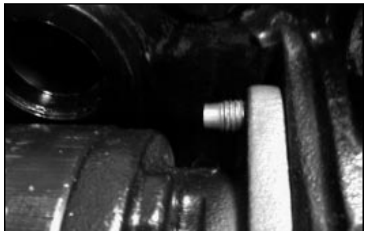
Photo 5. Starter-Bellhousing Bolt With Threads Ground Off To Form a Pilot.
