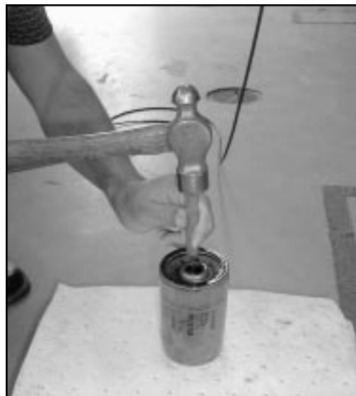
Photo 3: Punching the bottom of the oil filter.
