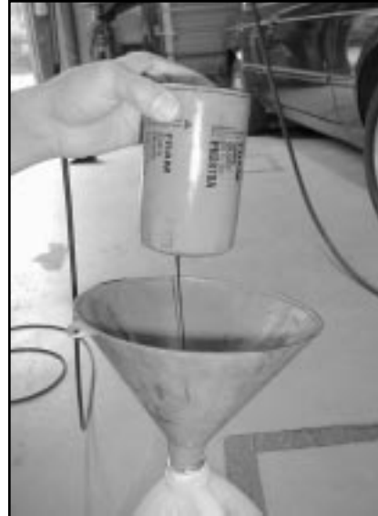
Photo 4: Steady stream of oil pouring out of the punched filter.
