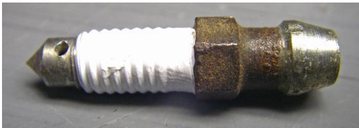
Photo #2 - Bleeder Screw Wrapped With Teflon Tape
