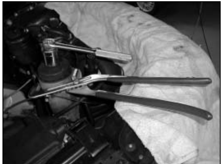
Photo 2: Removing The Oil Filter Canister Cover
